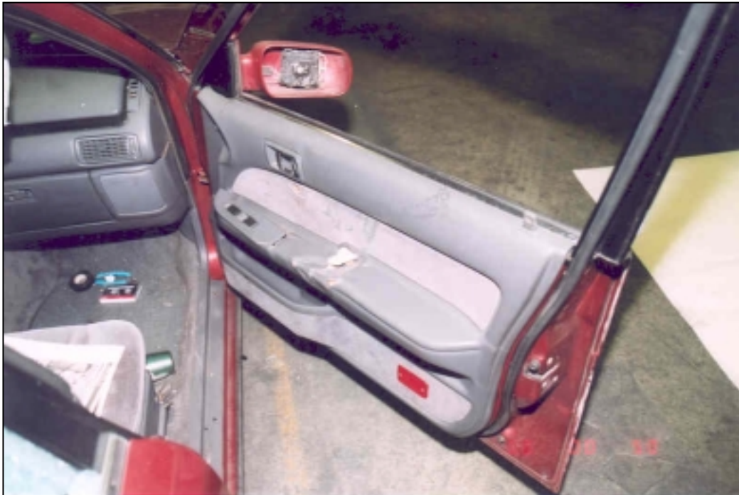
4 – Damage to Toyota’s front passenger door from impact with traffic signal pole with close up
